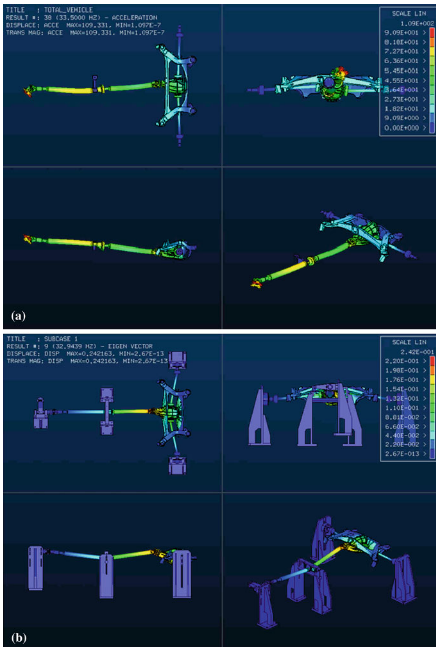
Fig. 8 Vibration results of the rear chassis system at 33 Hz a test and b calculation results
